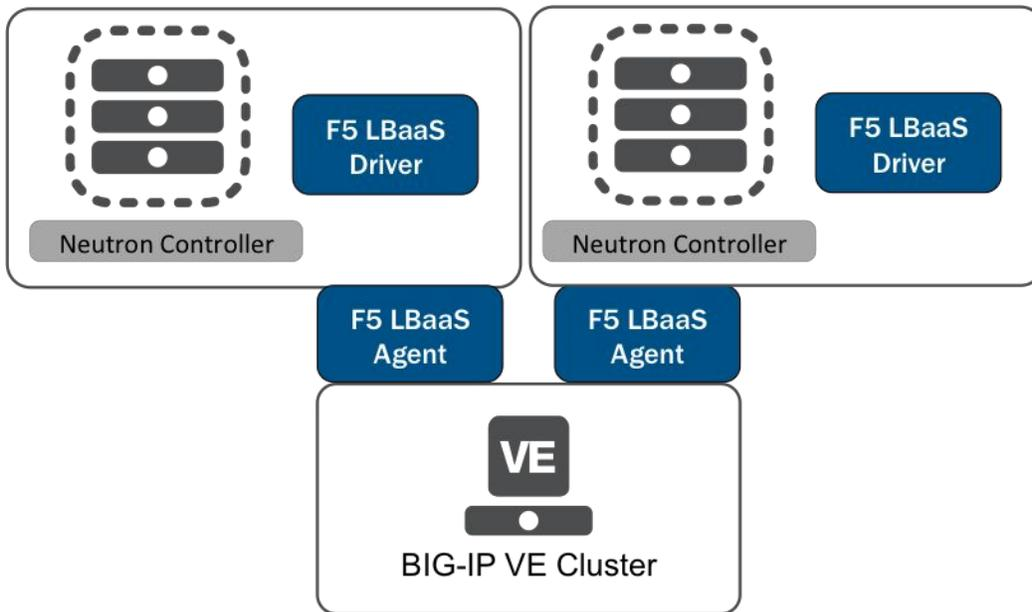
Figure 3: Multiple Neutron Controllers Connecting to a Single BIG-IP Cluster
