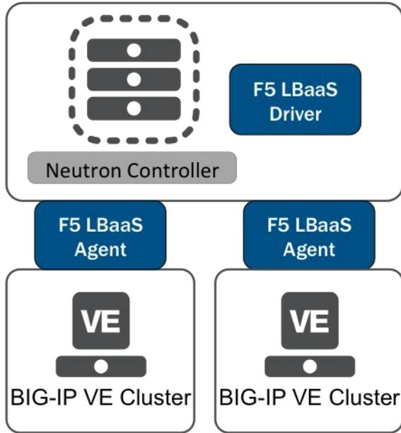
Figure 4: The F5 OpenStack LBaaS Plug-in orchestrating two different BIG-IP VE clusters from the same node..
